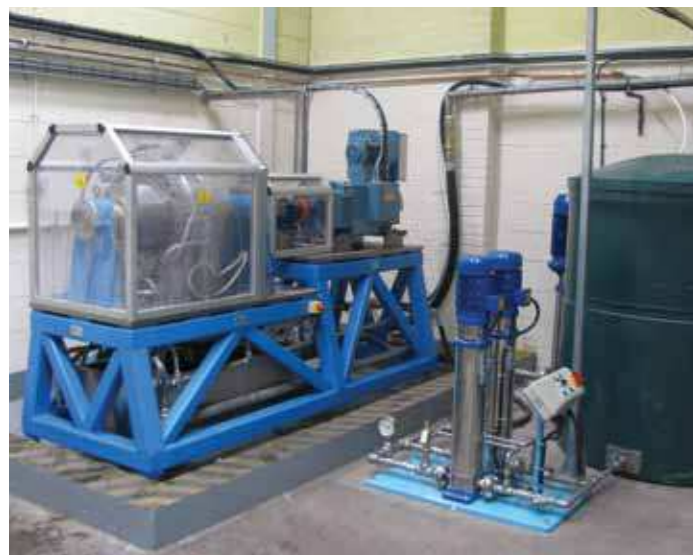
Specially commissioned test rigs at the James Walker Sealing Engineering and Materials Technology Centre allow testing of rotary seals under a wide variety of operational conditions
